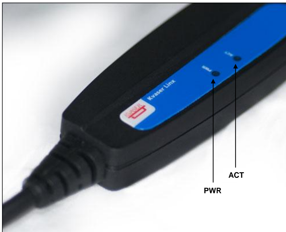
Figure 3: LEDs of the Kvaser Linx J1587.
