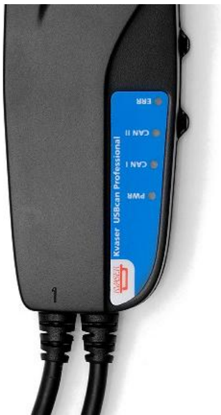
Figure 3: The CAN channels on Kvaser USBcan Professional.
