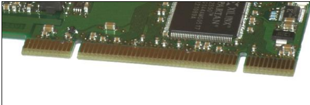
Figure 2. The 3.3 Volt and 5 Volt keyed board connector.
