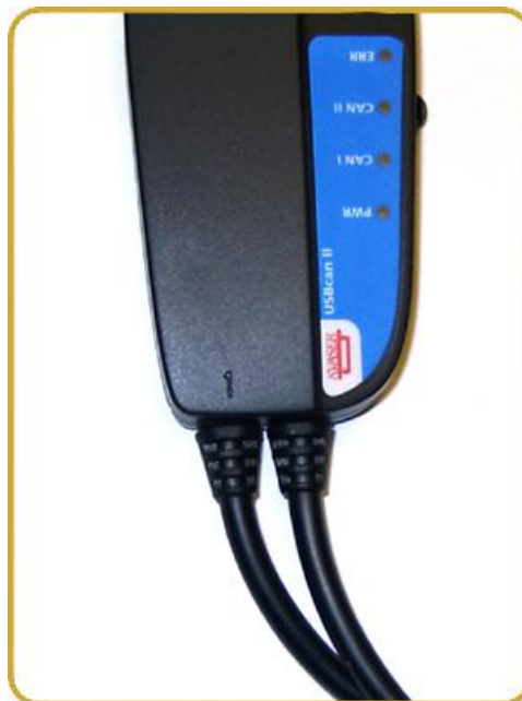
Figure 2. The channels on the USBcan II (channel 2 is not marked).
