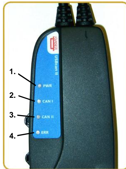
Figure 3. USBcan II LED configuration.
