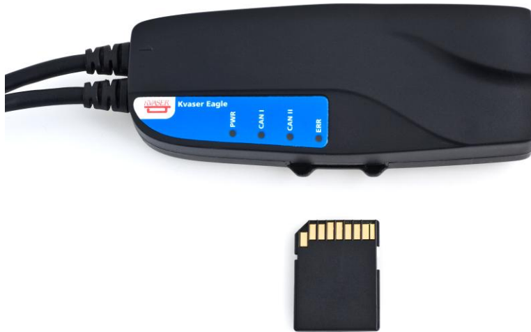
Figure 4: Inserting a Memory Card
