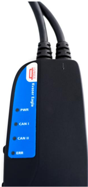
Figure 5. LEDs on the Kvaser Eagle
