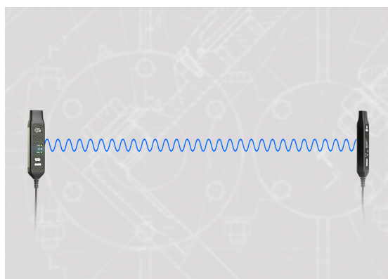
Figure 3: Radio units aligned in parallel is preferable.
