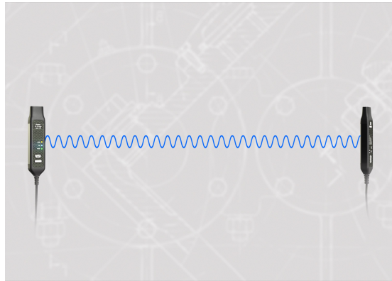
Figure 3: Radio units aligned in parallel is preferable.
