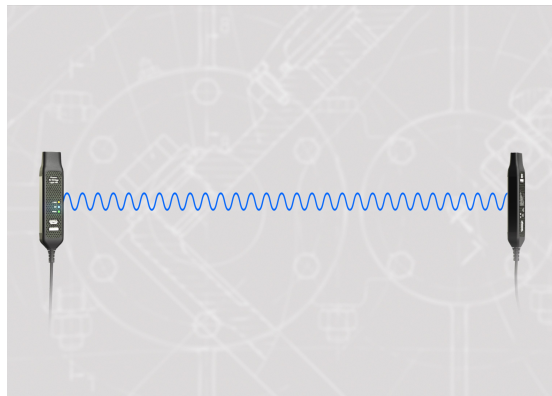
Figure 3: Radio devices aligned in parallel is preferable.
