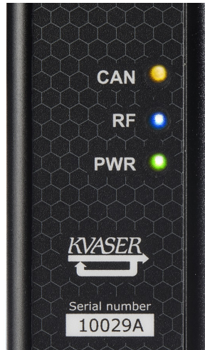
Figure 3: LEDs on the Kvaser Air Bridge Light HS.
