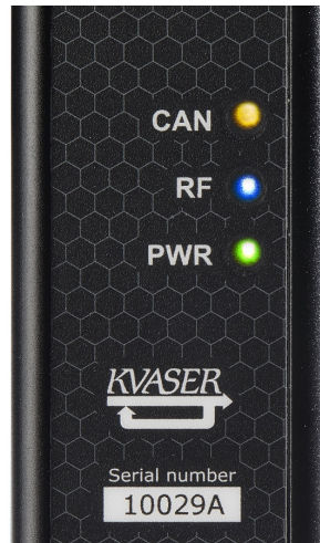
Figure 4: LEDs on the Kvaser Air Bridge Light HS.
