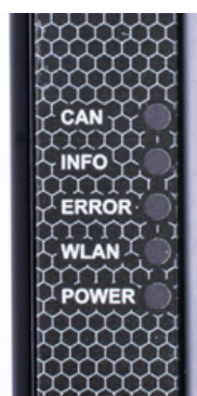
Figure 2: LEDs on the Kvaser BlackBird v2
