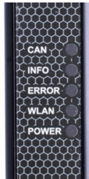
Figure 2: LEDs on the Kvaser BlackBird v2
