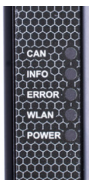
Figure 2: LEDs on the Kvaser BlackBird v2
