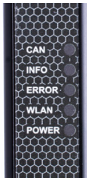
Figure 3: LEDs on the Kvaser BlackBird v2
