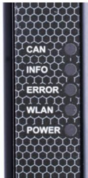
Figure 3: LEDs on the Kvaser BlackBird v2
