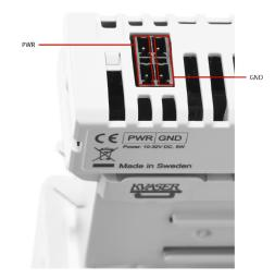
Figure 14: Power connectors on Base module.
