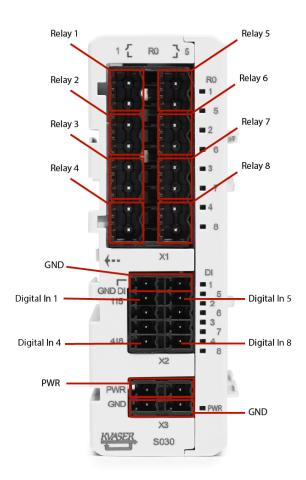
Figure 26: Relay add-on connectors
