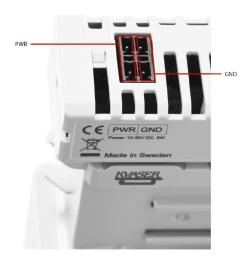
Figure 14: Power connectors on Base module.
