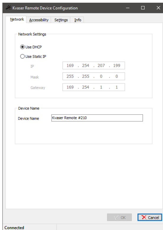
Figure 21: Kvaser Remote Device Configuration network settings
