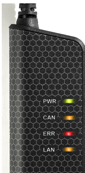
Figure 4: LEDs on the Kvaser Ethercan Light.
