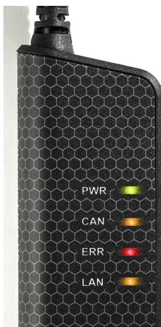
Figure 4: LEDs on the Kvaser Ethercan Light.
