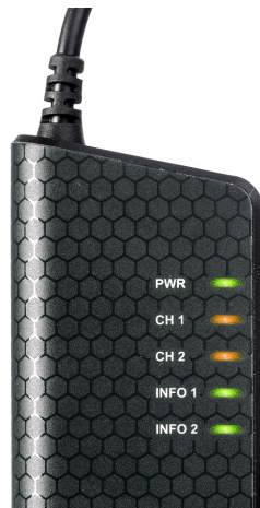
Figure 4: LEDs on the Kvaser Hybrid 2xCAN/LIN.
