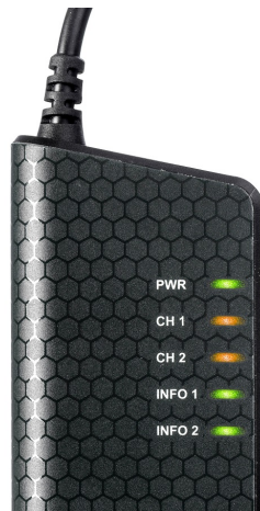
Figure 4: LEDs on the Kvaser Hybrid 2xCAN/LIN.
