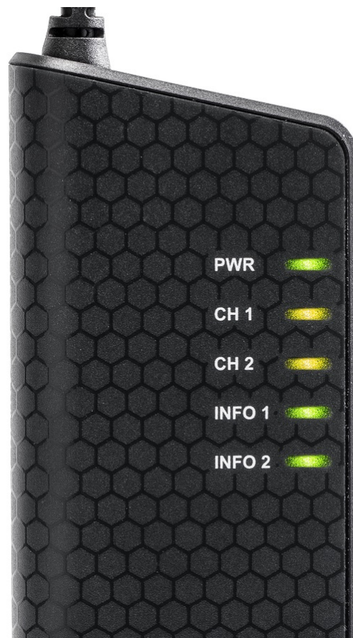
Figure 4: LEDs on the Kvaser Hybrid Pro 2xCAN/LIN.
