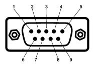
Figure 5: The D-SUB 9 connector pin numbers
