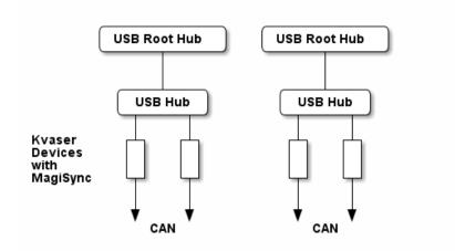
Figure 7: Not all devices are synchronized via MagiSync in this setup.
