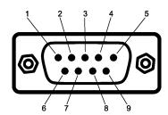
Figure 5: The D-SUB 9 connector pin numbers
