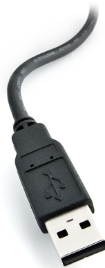
Figure 2: A standard USB type "A" connector.
