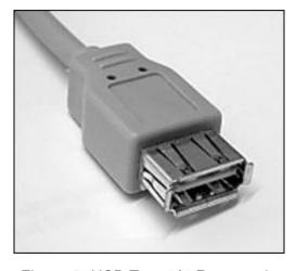
Figure 5: USB Type "A" Receptacle
