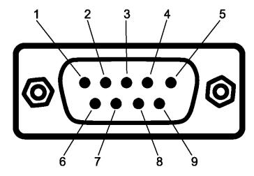
Figure 7: The D-SUB connector pin numbers
