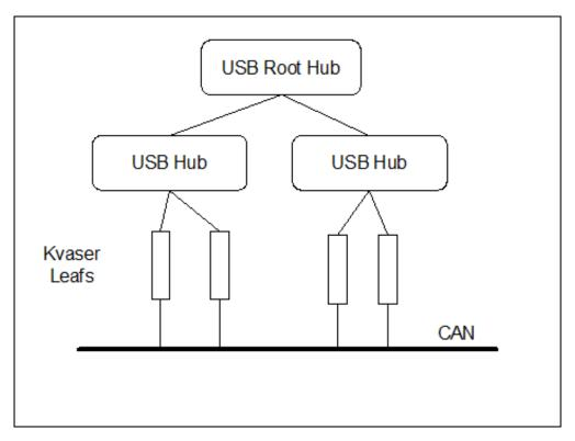
Figure 1: Kvaser Leaf syncronization. All devices are synchronized in this setup.
