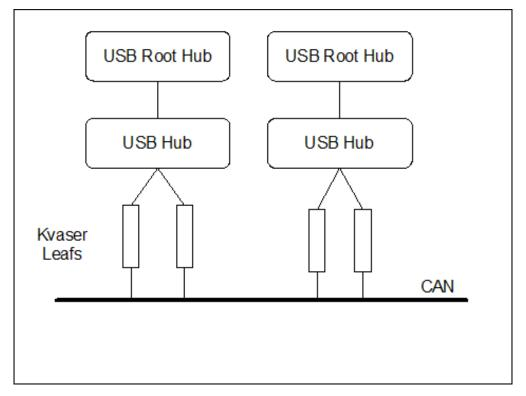
Figure 2: Kvaser Leaf syncronization. The devices are not synchronized in this setup.
