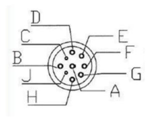
Figure 11: J1939-13 Connector pins
