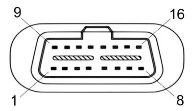
Figure 10: OBDII Connector pin Numbers
