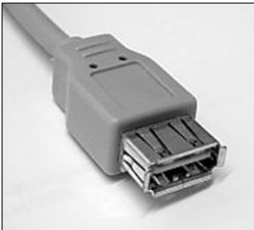
Figure 5: USB Type "A" Receptacle
