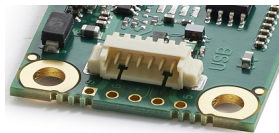
Figure 2: The USB connector.
