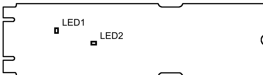
Figure 5: LEDs on the Kvaser M.2 PCIe 4xCAN.
