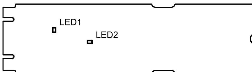
Figure 5: LEDs on the Kvaser M.2 PCIe 4xCAN.
