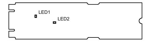
Figure 5: LEDs on the Kvaser M.2 PCIe 4xCAN.
