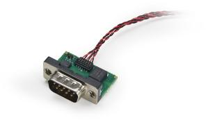
Figure 6: 9-pin D-SUB CAN connector.
