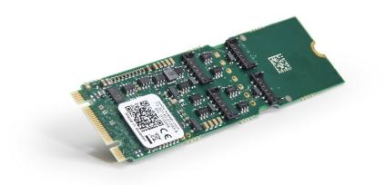
Figure 2: M.2 card of Kvaser M.2 PCIe 4xCAN
