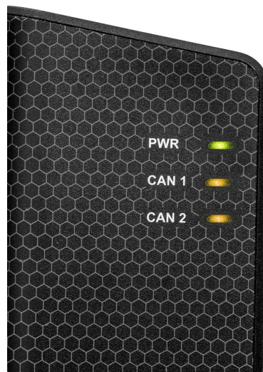
Figure 5: LEDs on the Kvaser Memorator 2xHS v2.
