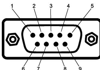
Figure 4: The D-SUB 9 connector pin numbers
