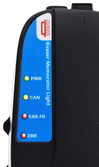
Figure 3: LEDs on the Kvaser Memorator Light HS v2.
