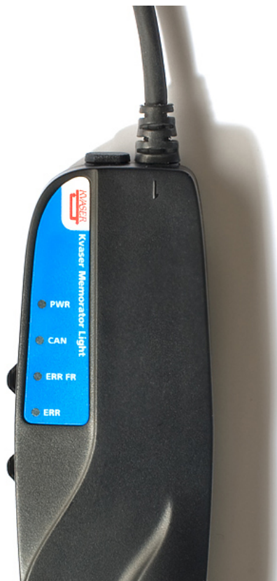
Figure 3: LEDs on the Kvaser Memorator Light
