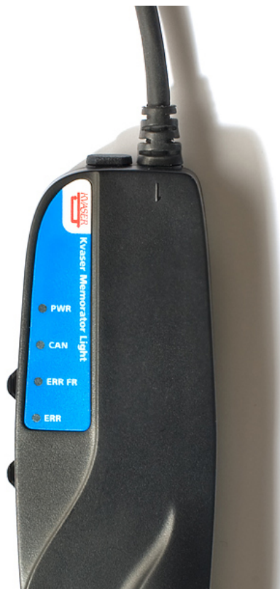
Figure 3: LEDs on the Kvaser Memorator Light
