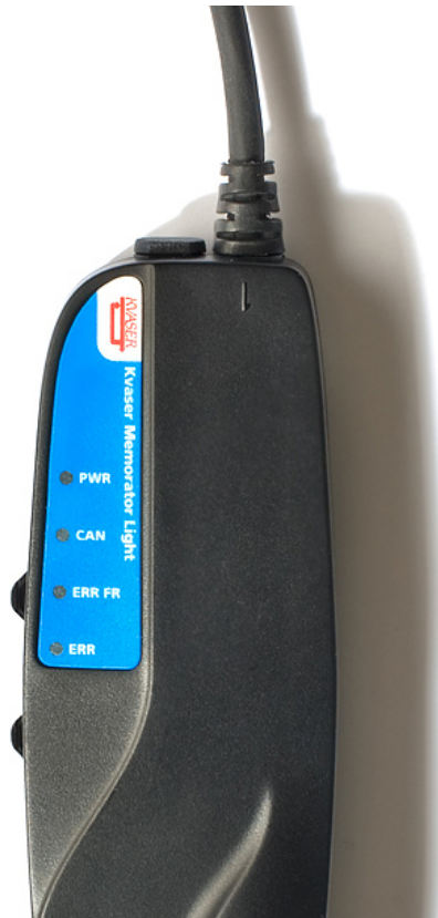
Figure 3: LEDs on the Kvaser Memorator Light
