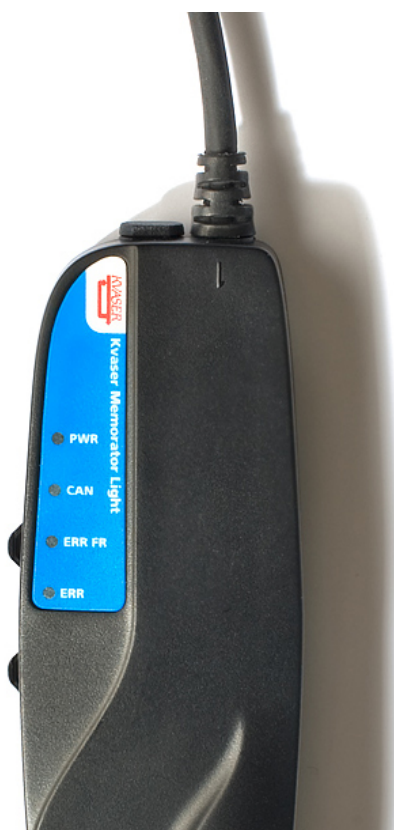
Figure 3: LEDs on the Kvaser Memorator Light
