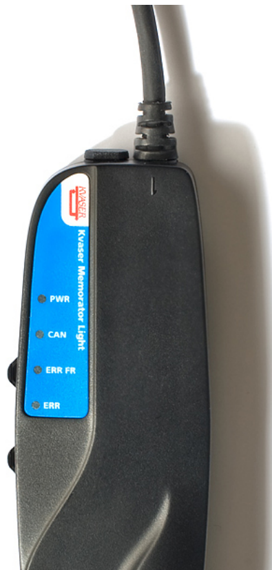
Figure 3: LEDs on the Kvaser Memorator Light
