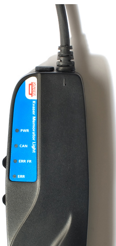
Figure 3: LEDs on the Kvaser Memorator Light
