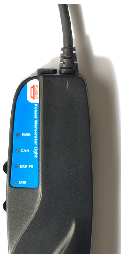
Figure 3: LEDs on the Kvaser Memorator Light
