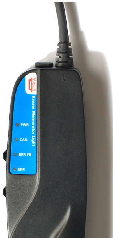
Figure 3: LEDs on the Kvaser Memorator Light
