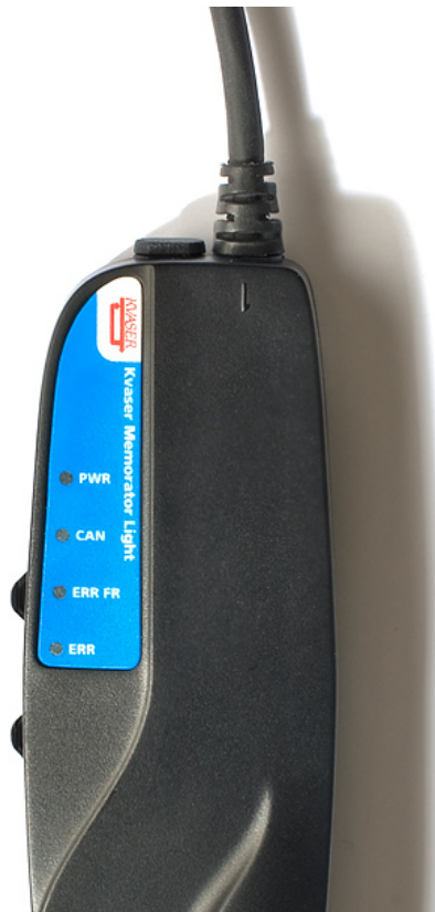
Figure 3: LEDs on the Kvaser Memorator Light
