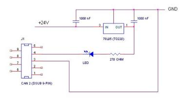
Figure 9: Sample circuit for connecting a LED to the External trigger output.
