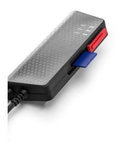
Figure 4: Inserting SD card into the Kvaser Memorator Pro 2xHS v2.
