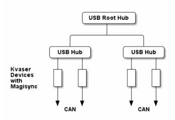
Figure 11: An example setup where all devices are synchronized via MagiSync.
