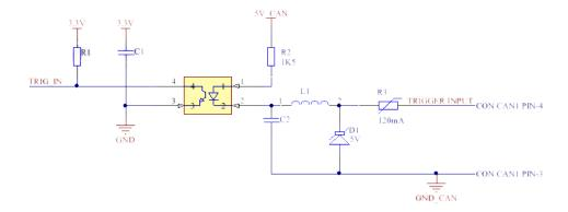
Figure 8: The External trigger input inside the Kvaser Memorator Pro 2xHS v2.
