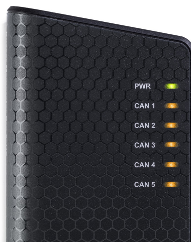
Figure 5: LEDs on the Kvaser Memorator Pro 5xHS.
