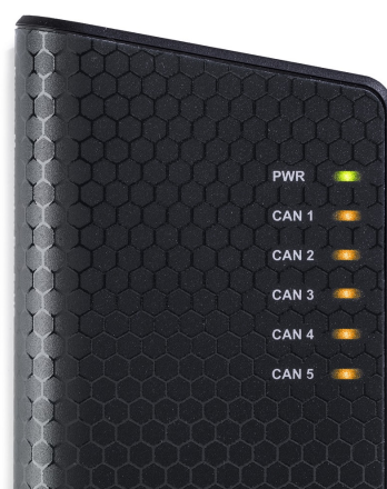
Figure 5: LEDs on the Kvaser Memorator Pro 5xHS.
