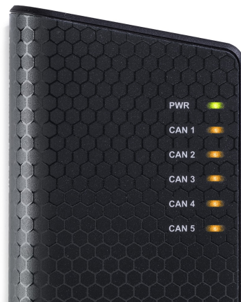
Figure 5: LEDs on the Kvaser Memorator Pro 5xHS.
