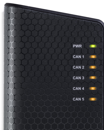
Figure 5: LEDs on the Kvaser Memorator Pro 5xHS.
