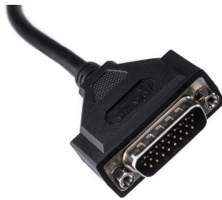
Figure 3: CAN connector on Kvaser Memorator Pro 5xHS
