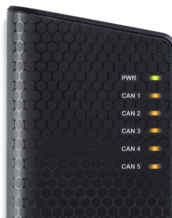
Figure 5: LEDs on the Kvaser Memorator Pro 5xHS.
